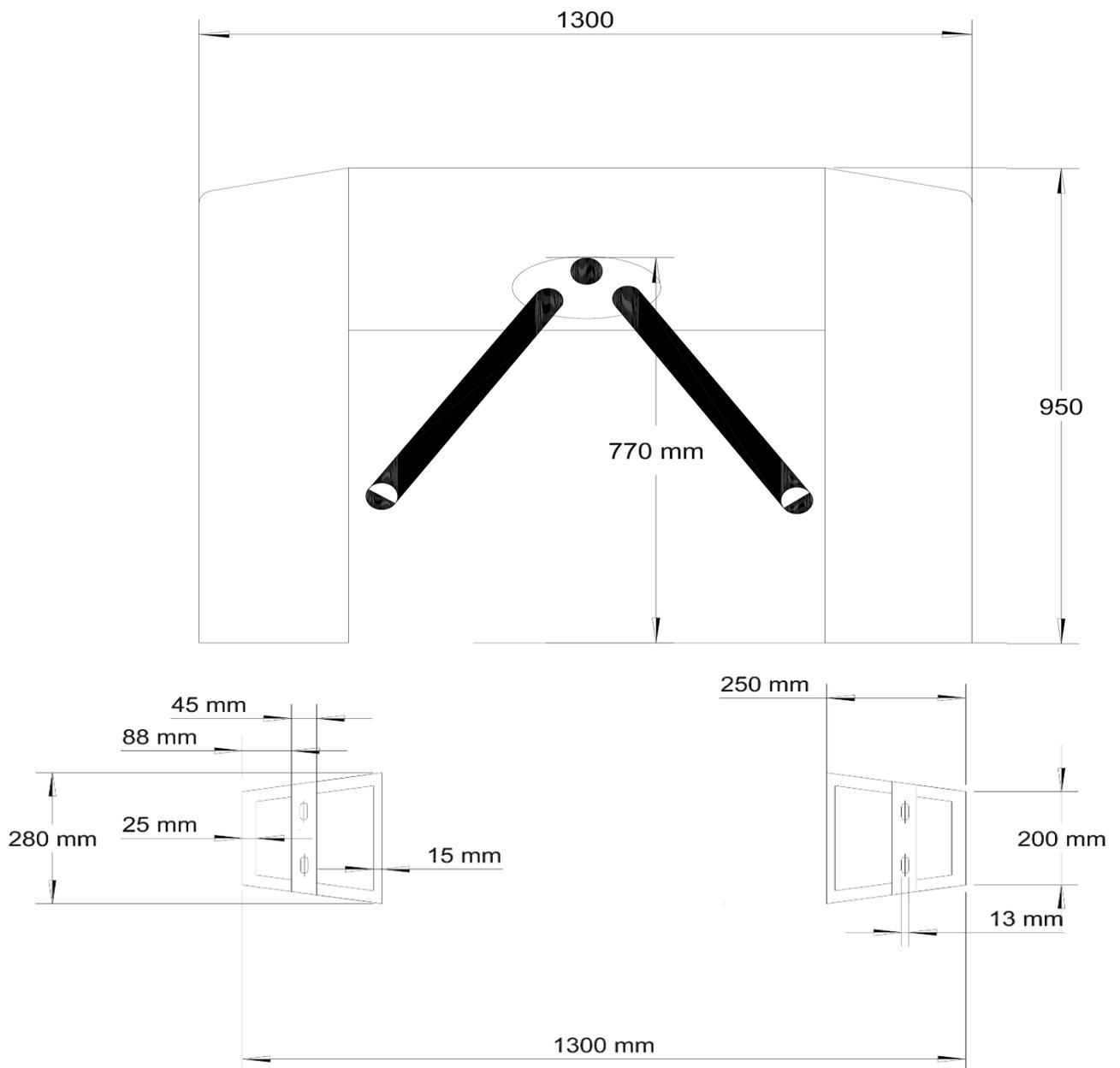
**NOTE:** The concrete pad should be 20Mpa (min) 150 mm thick, cured for 7 days on a suitably compacted foundation. Hold down anchors (4) to be 12mm dia x 100mm into the concrete.
