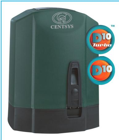
The D10 sliding gate operators use a high torque 24vdc motor, coupled to a robust gearbox that provides an automation system that is fast, powerful, easy to set up and fitted with battery back up.
