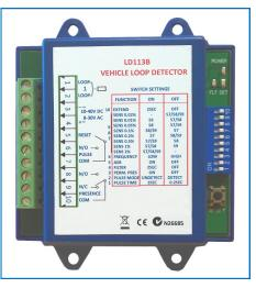
Loop detectors are most often used to open or prevent the closing of boom gates, doors or sliding gates.
