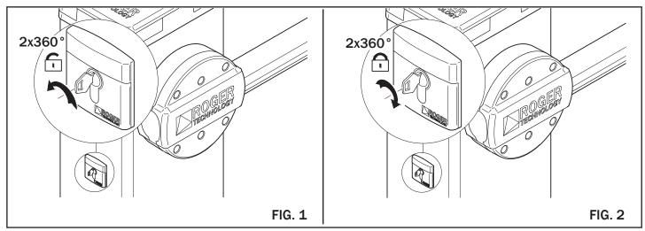
In some situations, such as in the event of a power outage or scheduled or extraordinary maintenance, it is necessary to release the automation. The operation of the release of the automation must be carried out when the boom is is stopped in the closed position (horizontal). Moreover, ensure that at the time of release, no person, animal, item or vehicle is passing by or stopped within range of automation.
