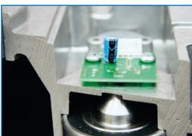
The advanced innovative and precise Absolute Encoder is assembled on the slow shaft of the motor. It monitors the safety sensing circuit hundreds of times a minute allowing for instant reverse of the boom pole.
